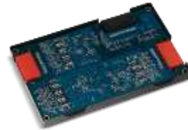
Battery Management System (BMS)
