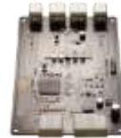
Battery Management System (BMS)
